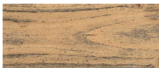
Untreated or conventionally oil-treated wood without UV protection
